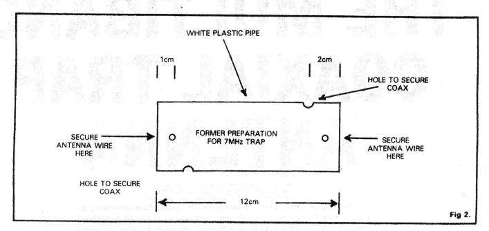
on and connected as in **Fig. 3.** This now dipped at 6.5 MHz, so the centre turns of the coax coil were spread with plastic spagetti, until resonance at 7 MHz was achieved.
